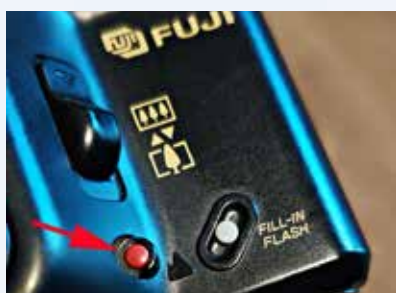
Fuji TELE CARDIA SUPER infinity focus button
