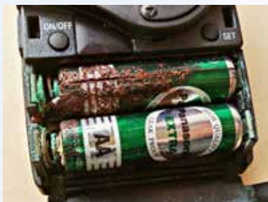
Extreme corrosion in battery compartment
