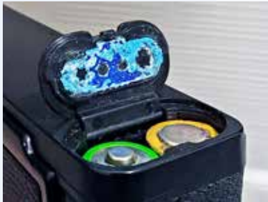
Corroded battery compartment cover
