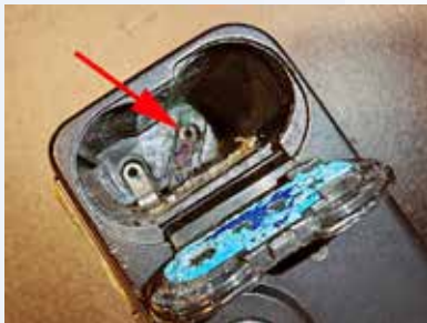
Corroded terminal inside camera
