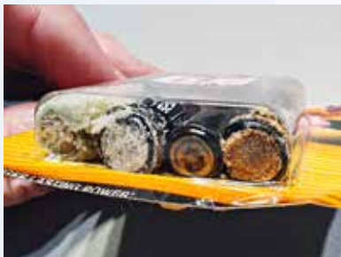
Leaking alkaline batteries in packet
